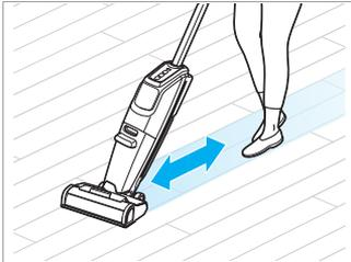
**6.** For best results, move machine forward to wet floor and backward to extract water.
