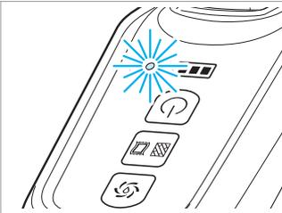
**7.** If the dirty tank is full, dirty tank indicator light will illuminate on the display. Empty the tank.
