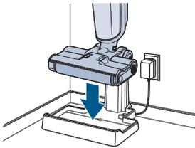
**1.** Place machine on docking station. Make sure clean water tank has cleaning formula and dirty water tank is empty.
