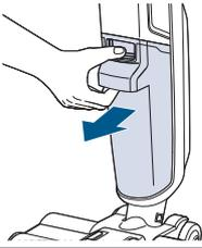
**1.** Press button on top of tank, grab front handle and pull tank out.
