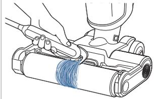
**9.** Use hook on cleaning tool to remove debris from brush roll.
