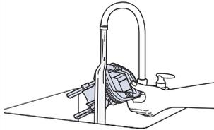
**5.** Wash filter with warm water and mild detergent. Rinse bottom of tank cover. **Note:** Filter must be completely dry before reinstalling.
