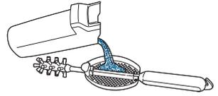
**3.** Use clean-out brush to strain debris while pouring into utility sink or similar waste water receptacle. Dispose of debris in trash and rinse tank.
