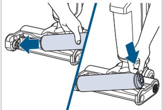
**12.** Place end of brush roll into left side of foot. Press brush roll tab down so it locks into place.
