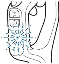
**4.** Dirty water tank indicator will flash red when tank is full or removed.
