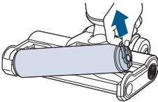
**7.** Pull brush roll tab to remove. Pull black tab to remove brush roll filter (behind brush roll).
