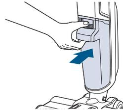
**15.** Insert bottom of tank first. Push top in until tank clicks into place.
