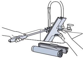
**8.** Hand wash brush roll, window and brush roll filter. Scrub parts with cleaning tool.
